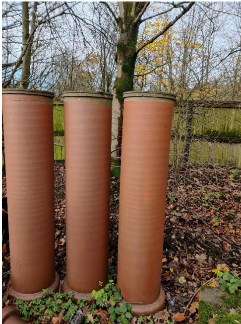
Figure 2: Surplus pipe sections (450mm dia.)
